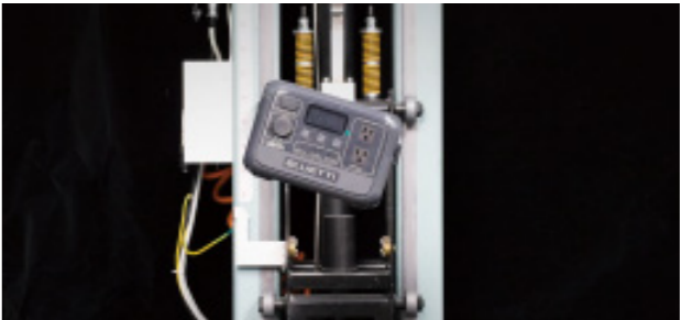
Shock Resistance Test Peak acceleration of 150 m/s, demonstrating resilience to high-impact shocks.
