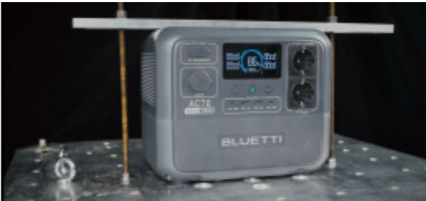
Transportation Scenario Restoration Test 100% recovery after vertical movement within 50mm for 30 minutes.
